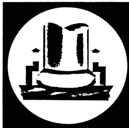
2. STUD LIFTS AND ARC IS DRAWN.
