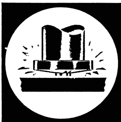
3. STUD FORCED INTO MOLTEN METAL.
